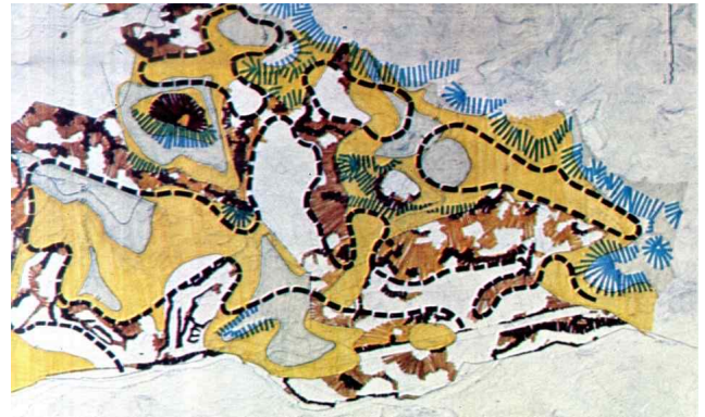
Figure 13. The Buildable Areas Calculated from the Geological Data of DPUA's Campus Plan
